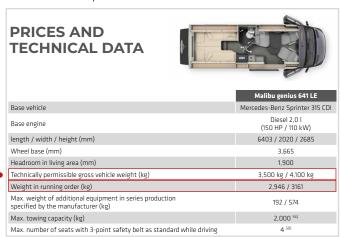
The technically permissible gross weight of the vehicle (e.g. 3,500 kg) must not be exceeded under any circumstances while driving. If the vehicle exceeds the technically permissible gross weight while driving, this constitutes a regulatory offence which may be punishable with a fine. We therefore urgently advise you to check this before each journey and ensure that you and your vehicle do not exceed the technically permissible gross weight (e.g. 3,500 kg).
